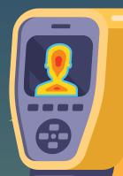
Thermal imaging cameras help reveal the areas of your home where poor insulation or air leaks are wasting energy and money and making your home less comfortable.
